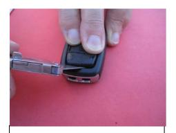
Using a Stanley knife, gently lift worn buttons pad and remove it from the top part of your remote.
