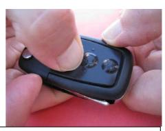
Place a new silicone pad over top part of your remote. Use rolling motion when positioning pad in grooves and press firmly till pad "engages" with hard shell all around edges and in the middle. If a new pad does not sit properly, remove it, clean grooves again and re-fit it. DO NOT USE any lubricants or detergents for cleaning grooves as it will affect firm seating of a pad.
