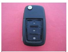
After removal of the old buttons pad, your remote should look like the one in the picture above, free of any old rubber pieces and dirt.
