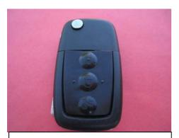
Your refurbished remote should look like the one in the picture above, with pad sitting firmly and flat all around edges and in grooves above and below middle button.
